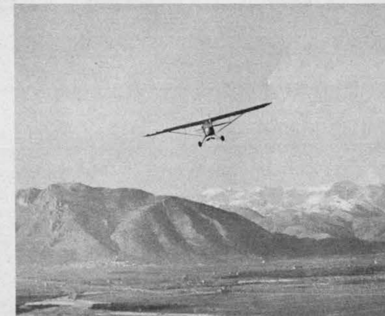
High wing braced with struts, and fixed landing gear make the L-4 Grasshopper look archaic. Head-on view of ex-Piper Cub circling over the Volturno River valley shows shock pads on landing gear struts.
